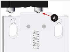
If the wiper blade is too high, remove the jet wiper assembly and turn the adjustment thumbscrew (A) clockwise. Reinstall the jet wiper and return to step 5.
